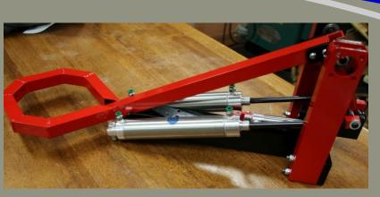
found that the pistons actuated slowly, and our distance actually decreased. The design we have decided to use has pistons (no springs) and ballast tanks to supply the needed influx of air.
